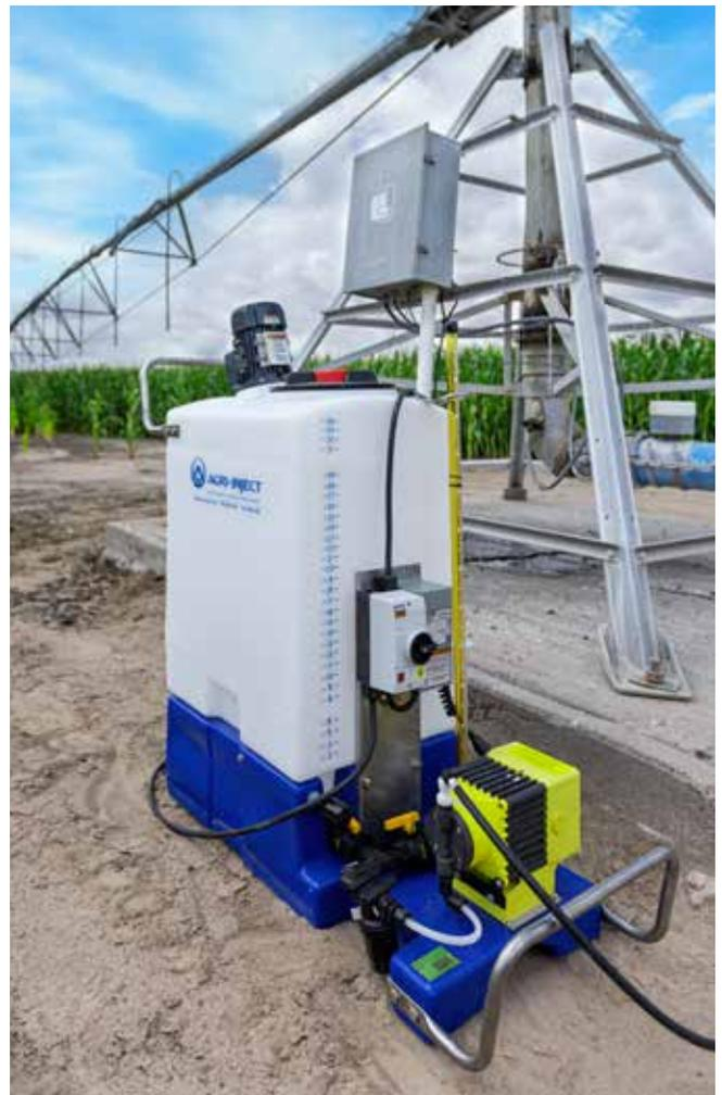
Agri-Inject’s Insectigator™, prior to redesign, in its natural habitat: integrating with a center pivot irrigation system to deliver crop-saving chemicals precisely where needed.
